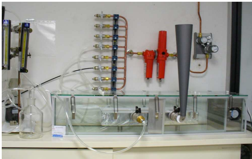
Figure 1 : Emission chamber with specimen
